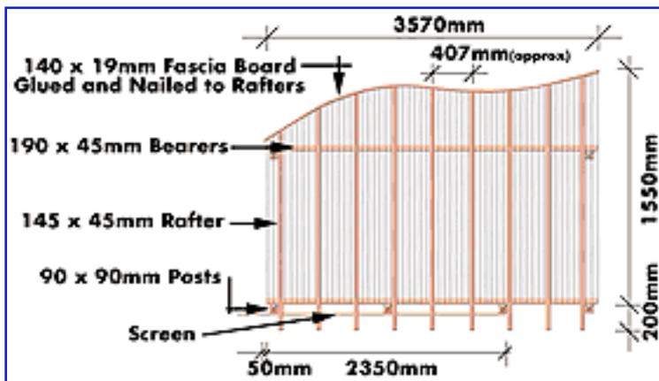
**Step 4** Rafters were fixed at 400mm centres on top of and perpendicular to the bearers. A decorative end to each rafter was created by removing one small corner of the rafter. Rafters were skew nailed to bearers ensuring the ends are in line. Battens were nailed to the top edge of and perpendicular to the rafters to accommodate the roof.
