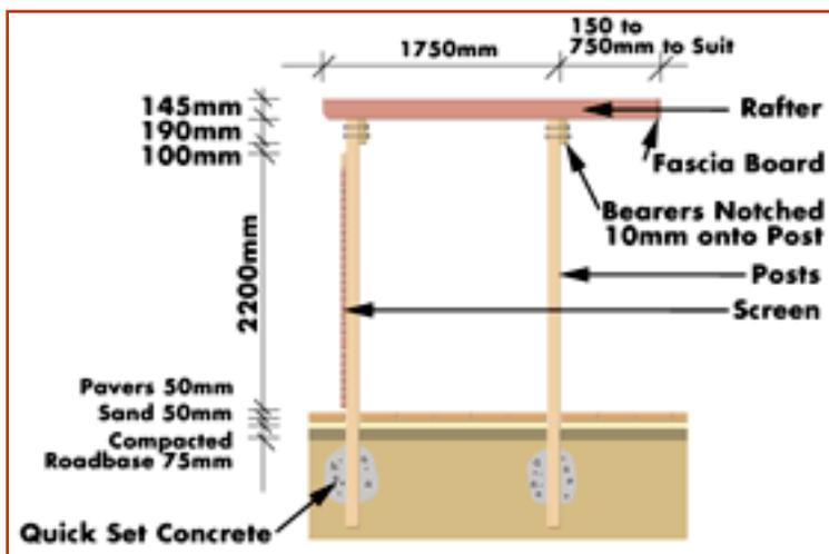
**Step 2** The posts were placed into the holes. Each hole was 1/3 filled with water and then filled with rapid set concrete to about 100mm below the top of the hole. More water was added to ensure the concrete would set. The concrete was allowed to set before proceeding further.
