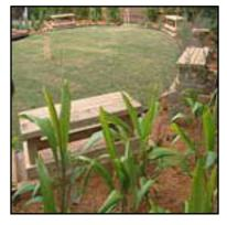
**Bench seats:** Scott knocked up some simple bench seats from which to enjoy the entire garden. Short lengths of treated pine posts (H4, 90x90) support rails (90x45mm) nailed in place. The bench top is simply wide boards (140x45mm) screwed in place with a 10mm gap between each piece.
