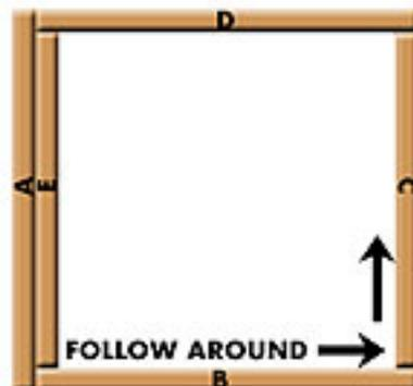
(point E on the diagram) and continue working in an anticlockwise direction. Note: No two pieces of sleeper will be the same length as the square is getting smaller (each piece is the width of a sleeper shorter than the one before it). Measure and cut one piece of sleeper at a time. If the last space is too narrow for a full sleeper, cut it to fit.
