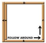
**Step 2** Form a frame by laying out sleepers for the four sides (A, B, C, D in the diagram above). All corners should be at right angles (90°). Drive treated pine pegs at 500mm intervals along the outside edge of the framing sleepers and nail these pegs to the sleepers.
